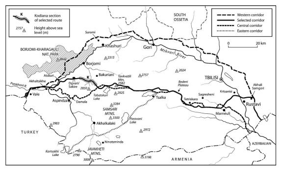
**Figure 2.1** Alternative pipeline routes through Georgia. Map prepared by Ailsa Allen, School of Geography and the Environment. Reproduced by permission of the University of Oxford
